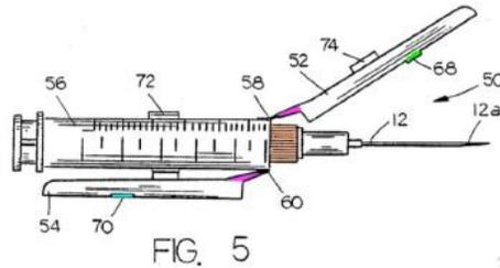
Pet. 28. Figure 4 depicts “an elevational view of a syringe with the safety cover of [Norelli’s] invention thereon, the safety cover in a secured, closed condition.” Ex. 1015, 3:23–25. Figure 5 depicts “an elevational view of a syringe with one jaw of [Norelli’s] invention being moved into a closed position.” *Id.* at 3:26–28.
