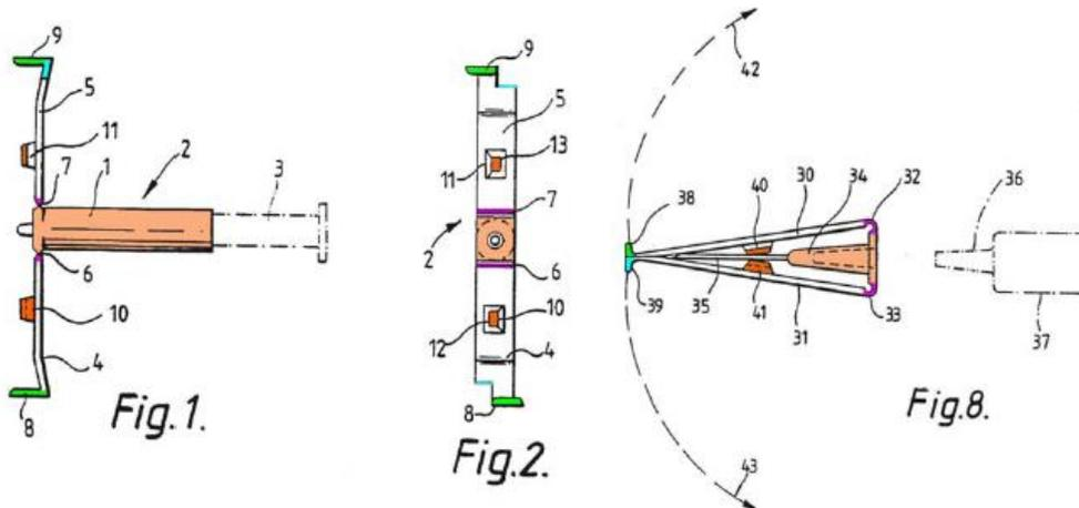
Pet. 31. These annotated figures show Cole’s device 2, with certain components allegedly corresponding to recited claim limitations colorized. With respect to the “substantially perpendicular” limitation of claim 1, RMS contends that “as stub outlets are known to be curved to provide fluid delivery at a perpendicular angle to the barrel of the syringe, the needle **35** may be substantially perpendicular to the delivery tube **36**.” *Id.* at 33. RMS continues that:
