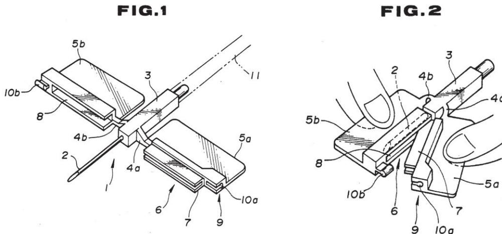
Figure 1 provides a perspective of an embodiment of Ishikawa's winged needle, and Figure 2 depicts the embodiment of Figure 1, during the process of covering the needle. *Id.* at 1:56–59. Ishikawa's winged needle 1 includes needle 2 attached at one end to base 3 and wings 5a, 5b attached to base 3 through arms 4a, 4b. *Id.* at 2:6–9. These components are made from an elastomeric material, such as synthetic rubber. *Id.* at 2:9–11. Base 3 is attached to flexible tube 11. *Id.* at 2:34–35.
