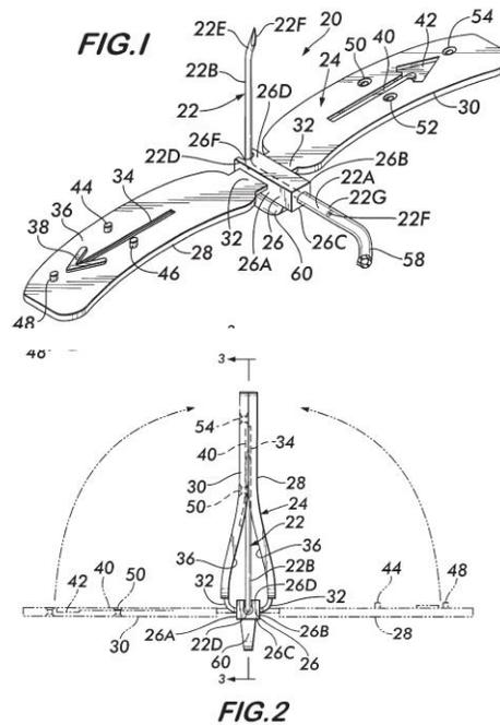
Figure 1 provides an isometric view of Sasso’s needle safety device in an open position, and Figure 2 depicts the same embodiment in a closed position. *Id.* at 3:34–41. As seen in Sasso’s Figure 1, Sasso’s mechanical fastener includes posts 44, 46, 48 that mate with apertures 50, 52, 54. Also as seen in Figure 1, distal end portion 22B is perpendicular to proximal end portion 22A.
